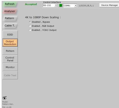
**Figure 6: Output Resolution in Analyzer Mode, Portable Version**
