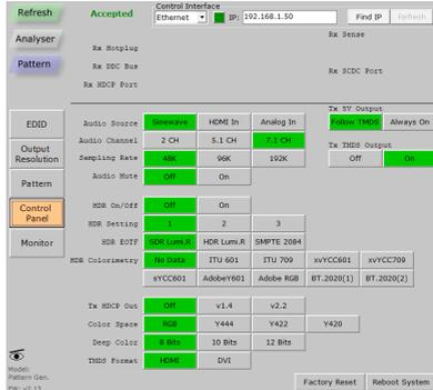
**Figure 9: Control Panel in Pattern Mode, Bench Version**
